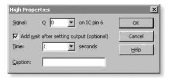
This will make the output connected to Q0 go high (if a bulb was connected, for example, the bulb would light up).
