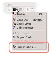
First of all, you need to tell GENIE which type of chip you are using. To do this, click on the Microcontroller button on the toolbar and choose Program Settings.
