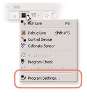
First of all, you need to tell GENIE which type of chip you are using. To do this, click on the Microcontroller button on the toolbar and choose Program Settings.
