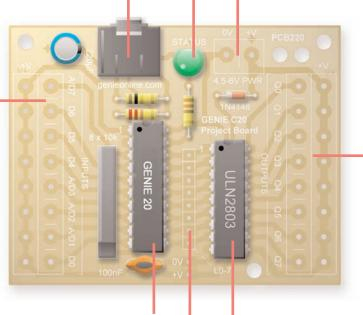
Medium-power outputs, controlled by signals **Q0** to **Q7**
